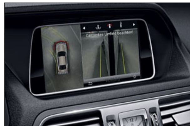
Parking package with 360° camera, incl. Active Parking Assist with PARKTRONIC
