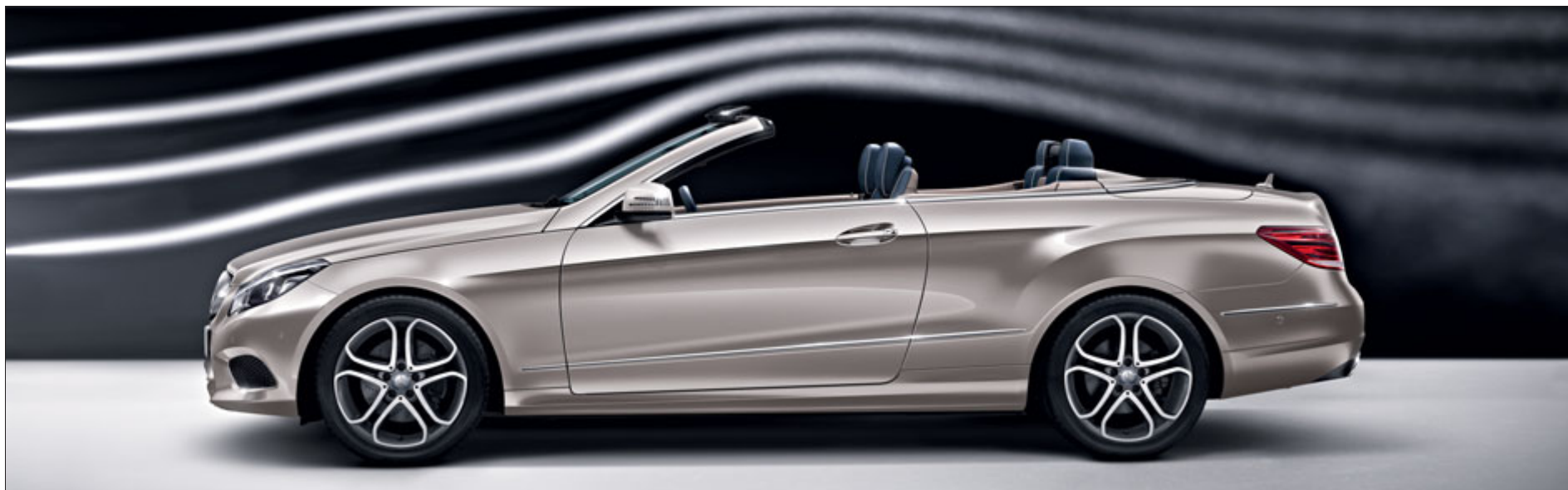
The enhanced AIRCAP system now reacts to the number of occupants and features speed-sensitive control
