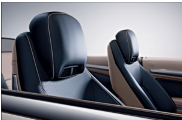
AIRSCARF neck-level heating at the front
